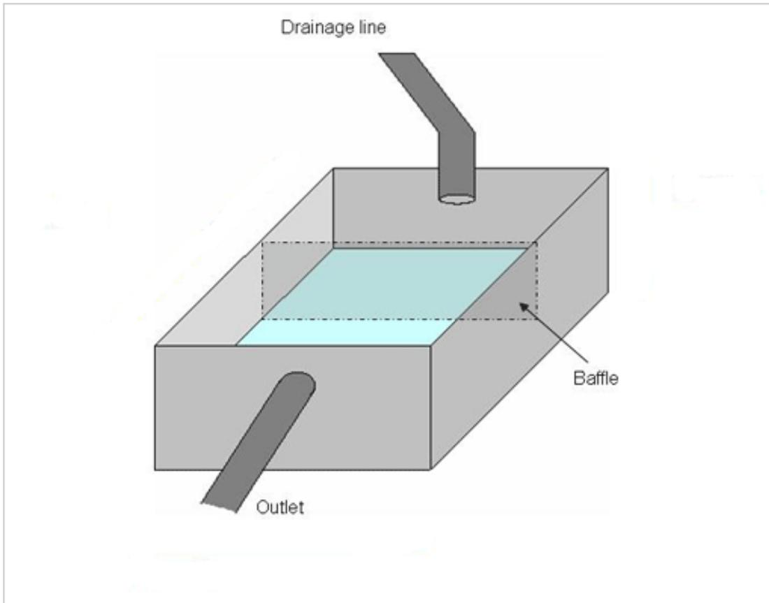
Schematic of a basic sediment trap. Not illustrated is the grated top of the trap which can be removed to recapture the accumulated sediments.
