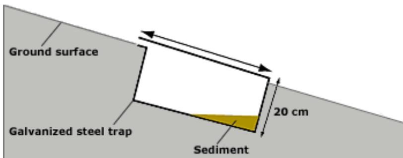
Schematic diagram illustrating the operation of the above driveway spanning sediment trap.
