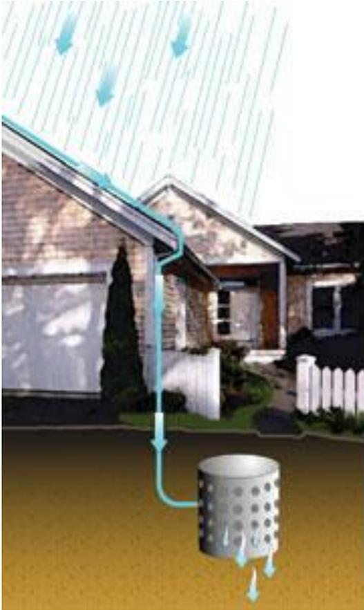
Stormwater infiltration systems allow stormwater to drip into the soil joining groundwater.
